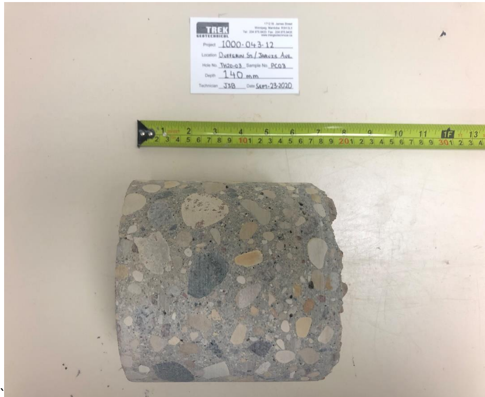
Photo 3: Pavement Core Sample at Test Hole TH20-03
