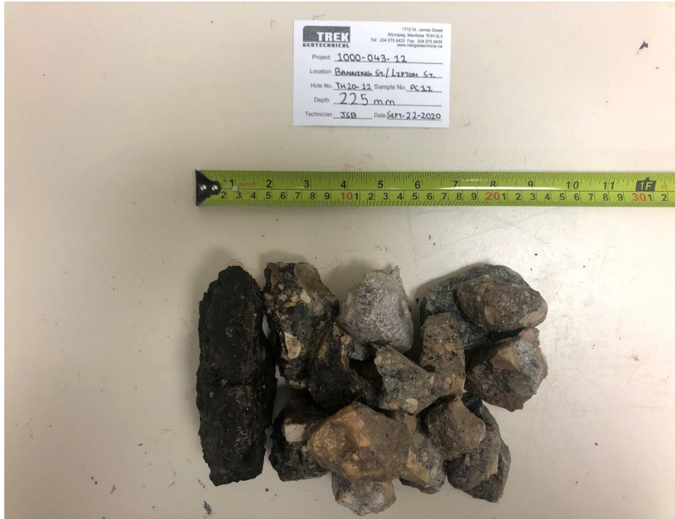
Photo 1: Pavement Core Sample at Test Hole TH20-12
