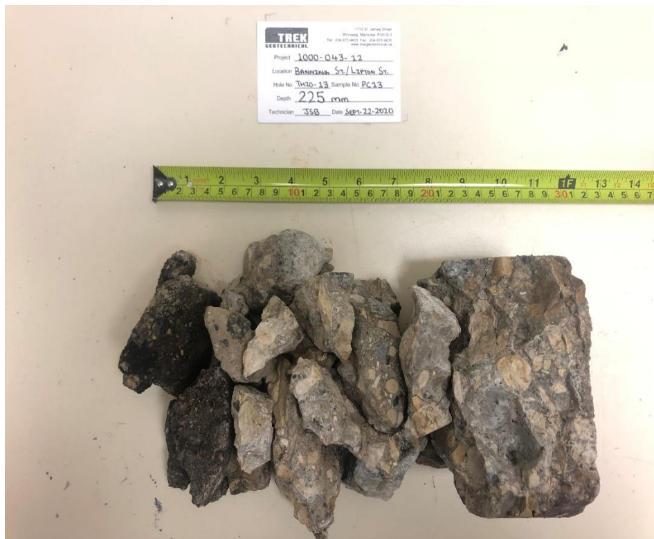
Photo 2: Pavement Core Sample at Test Hole TH20-13
