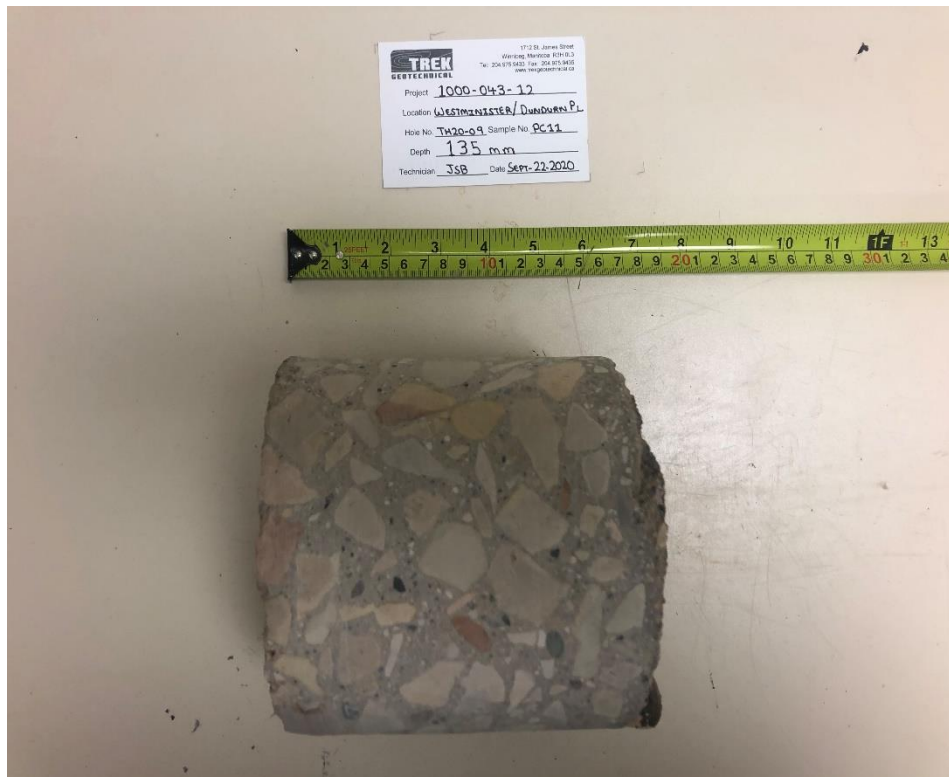
Photo 2: Pavement Core Sample at Test Hole TH20-09
