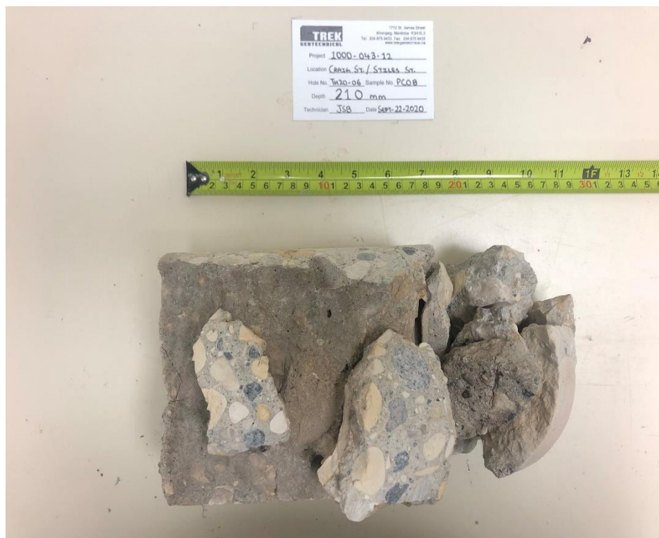
Photo 2: Pavement Core Sample at Test Hole TH20-06
