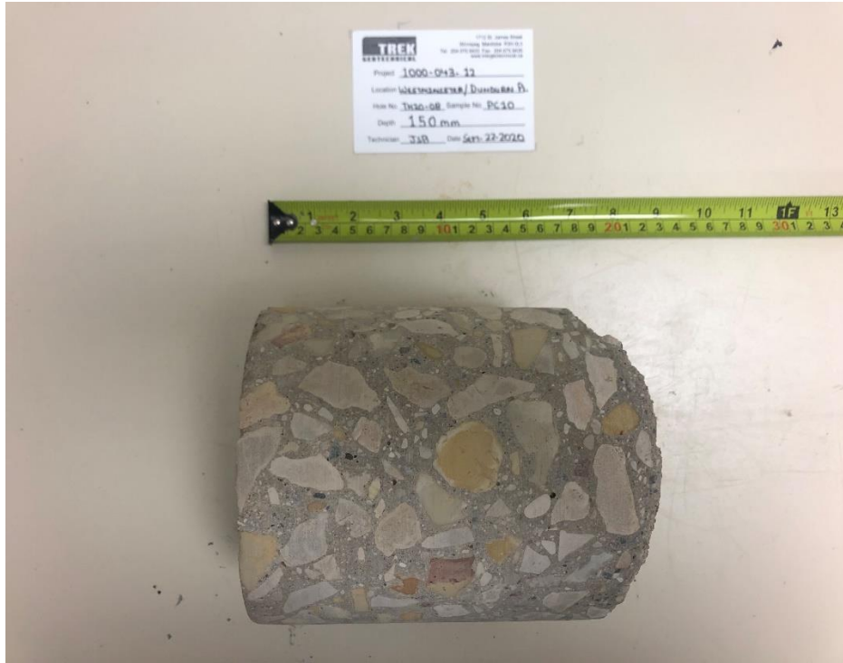
Photo 1: Pavement Core Sample at Test Hole TH20-08
